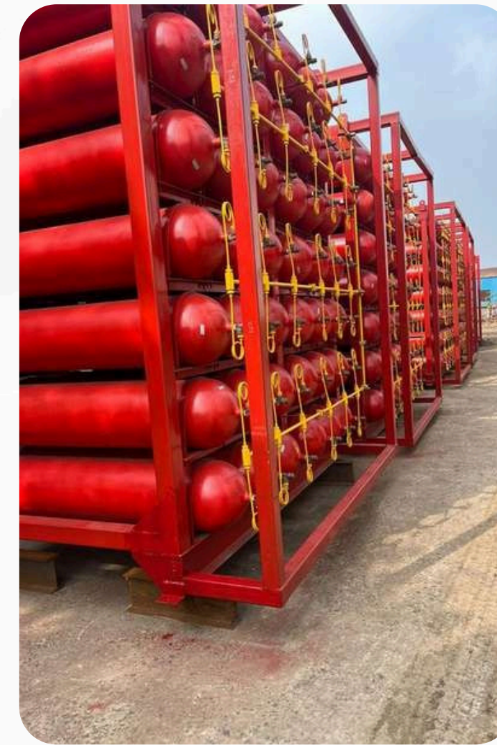
42 CYLINDER – 200 Bar– 67 Kg H2 Storage
